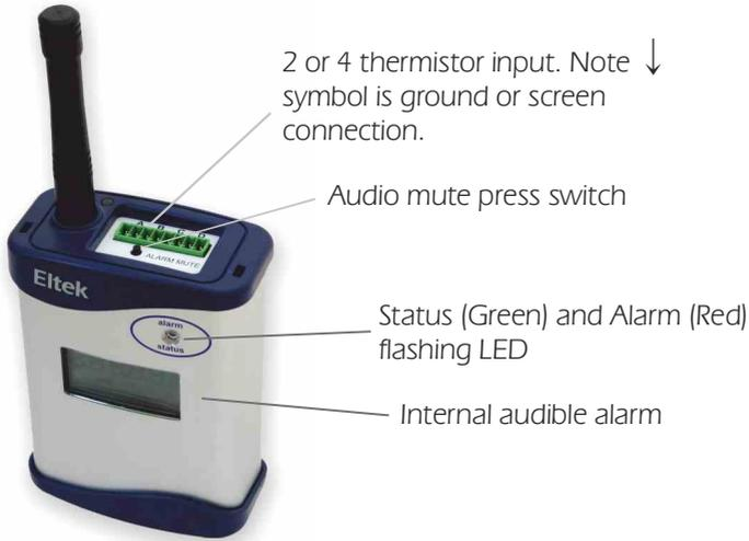
The GD32ALS and GD34ALS transmitters provide 2 thermistor or 4 thermistor/state inputs with visual and audible alarms for any input that exceeds a configurable threshold.
