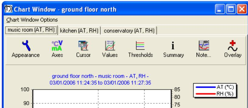
On any one chart you can only have two axes. Therefore you can only assign two parameters to any chart e.g. temperature and RH, with one assigned to the **Left axis** and the other to the **Right axis**.
